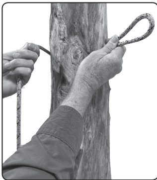
Figure 14 Wrap sewn-in loop end of tree tether around tree trunk.
