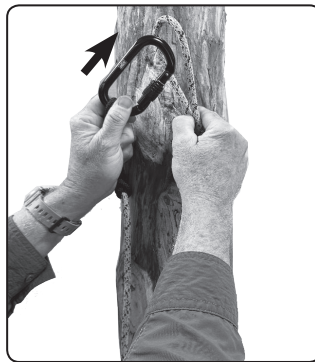
Figure 15 Slip locking carabiner end of line-man rope through sewn-in loop.
