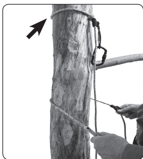
Figure 21 Install tree tether ABOVE obstacle and to the tree trunk.
