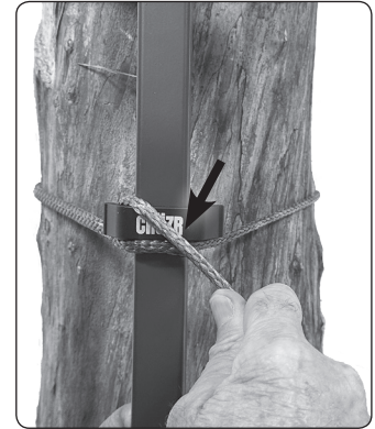
Figure 10 Pull connector rope ACROSS AND DIAGONALLY DOWN cleat face.
