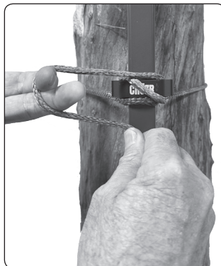
Figure 12 With your palm facing you, wrap the connector rope around index and middle fingers.
