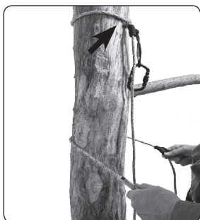
Figure 17 Install tree tether ABOVE obstacle and to the tree trunk.
