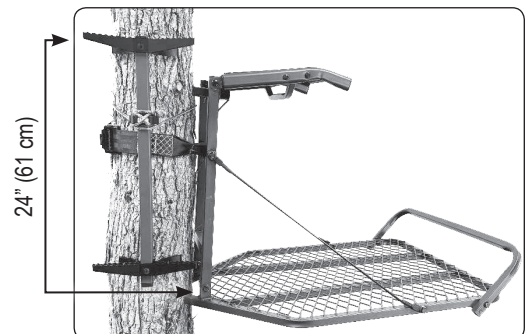
Figure 3 Install Solution Sticks™ a minimum of 24-inches above hang-on style treestand standing platform.
