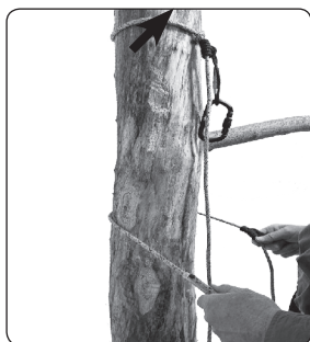
Figure 12 Install tree tether ABOVE obstacle and to the tree trunk.
