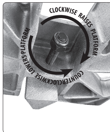
Figure 15 Adjust standing platform by rotating standing platform angle adjust clockwise or counterclockwise.
