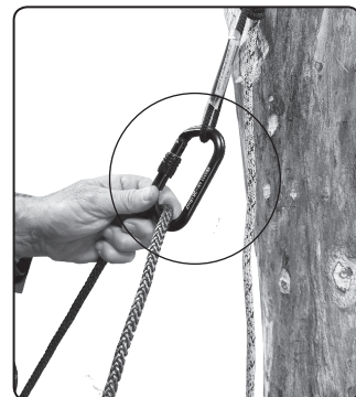
Figure 16 Attach locking carabiner to bridge.
