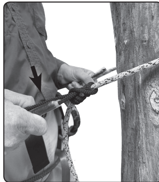
Figure 12 Lineman rope MUST BE at, or above waist level at all times.
