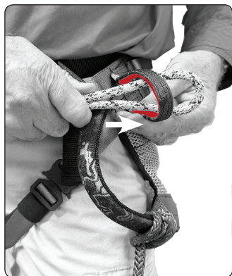
Figure 8 Slip sewn-in loop through lineman belt loop w/ red liner.
