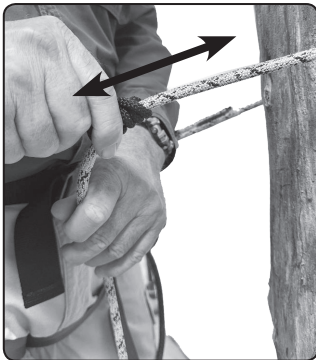
Figure 11 Slide locking carabiner prusik knot up and down to adjust distance from tree.
