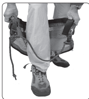
Figure 4 Step through the bridge.
