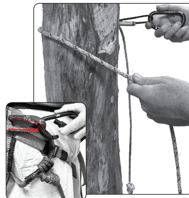
Figure 10 Wrap lineman rope around tree trunk and connect locking carabiner to lineman rope loop w/red liner.
