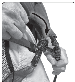
Figure 19 Pressure on waist area, slide bridge knots down.
