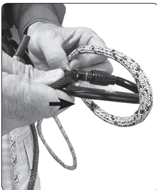
Figure 9 Slip locking carabiner end of lineman rope through sewn-in loop.
