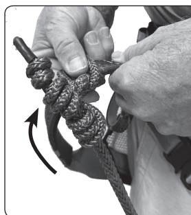
Figure 20 Pressure in leg area, slide bridge knots up.
